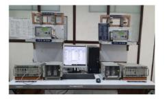
appreciate the advantages of Digital axle counters over conventional track circuits. Trainee will be able to know the advantage of HASSDAC over SSDAC in improving the reliability of the system.
